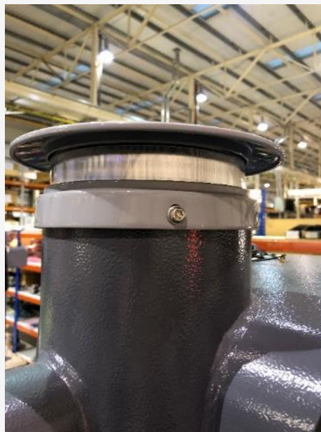
Figure 11 - LED on Tower
